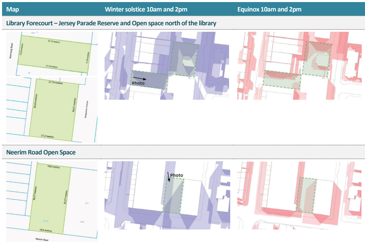
Figure 6 Library forecourt – Jersey Parade Reserve, Open space north of the library and Neerim Road Open Space – map and overshadowing diagrams
