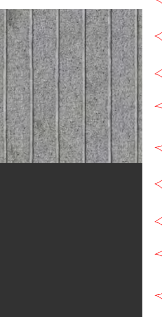
RENDERED FINISH WITH VERTICAL GROOVES; RENDER COLOUR TO MATCH COLORBOND 'MONUMENT'
