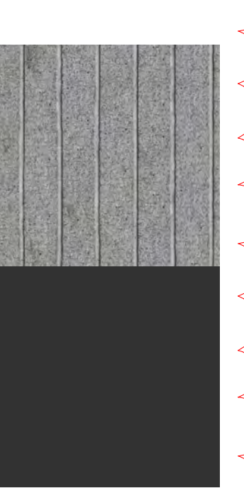
RENDERED FINISH WITH VERTICAL GROOVES; RENDER COLOUR TO MATCH COLORBOND 'MONUMENT'
