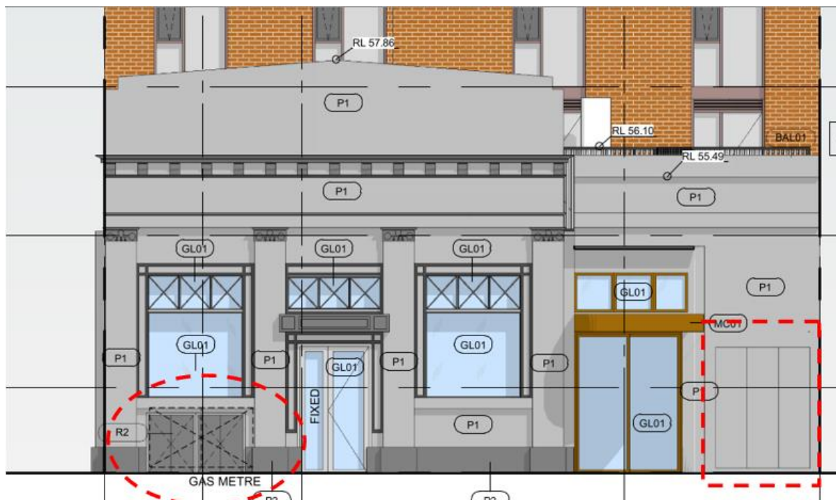
Figure 3 - Ground floor facade showing fire and gas services
