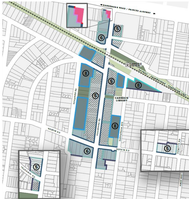
Figure 17. Building envelopes for the Carnegie 'Main Retail Precinct' (Source: Carnegie Built Form Framework, 'Figure 10: Main retail precinct building envelopes', p 42).
