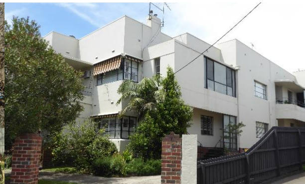
66-68 Riddell Street, Lowan Court Moderne/Functionalist style flats, concealed roof, render and clinker brick plinth, steel-framed windows, curved balconies, original fence
