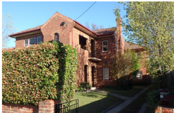
15 Stanley Street Durham Old English style, clinker brick with some tapestry bricks to openings, Tudor arches, original fence
