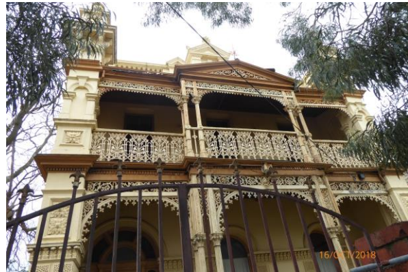
70 Orrong Road, Lisbon House (HO52) – 1889, Italianate style, two-storey, elaborate cast iron verandah with central pediment, and extensive use of rendered mouldings to wing walls (niches and floriated panels) and parapet (large brackets, urns, niches, etc.)
