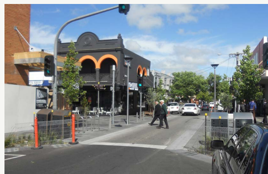
WIDER CROSSINGS: The provision of wider crossings of 4m to 6m or wider in locations with high flows reduces conflict and changes perceptions of space allocation.
