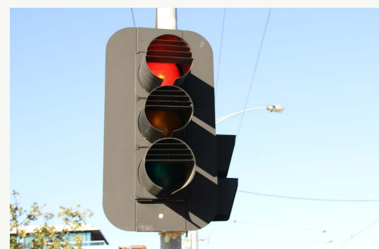
REST ON RED: Traffic signals sit on red until activated by a vehicle, while at all other times pedestrian signal sits on green.
