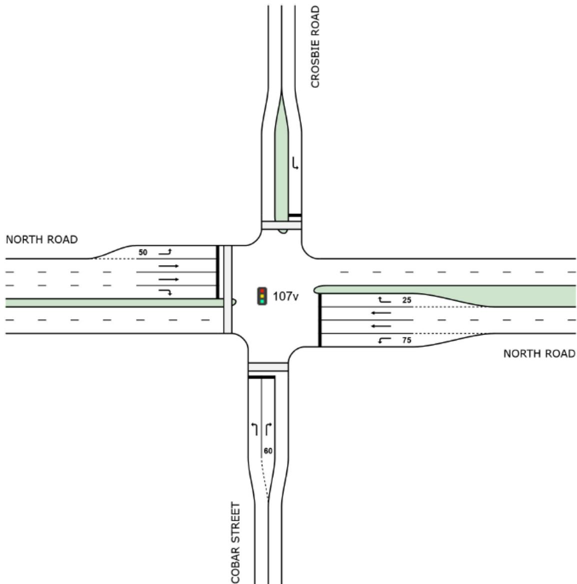
Subject to the pedestrian phase across Crosbie Road not operating when traffic is turning right out of Cobar Street, it is considered that appropriate regulatory signage and linemarking would be sufficient to achieve the desired outcome of minimising additional through traffic using Crosbie Road.
