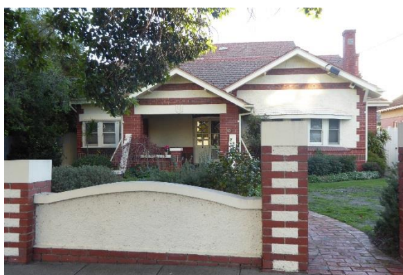
No. 26 – clinker brick head and soldier banding with extensive render and bow window (leadlighting)
