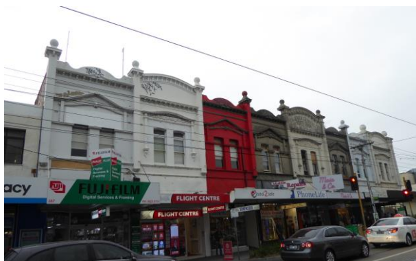
357-371 Glenhuntly Road Buckeridge's Buildings, 8 premises built in two stages – 1911 (eastern four) and 1914 (western four) Parapet with scalloped sections and orbs Render finish remains unpainted to nos 363 and 367 Sinuous floral decoration (Art Nouveau style) above paired windows, framed by thin fluted pilasters
