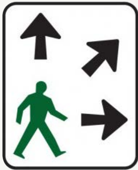
SCRAMBLE CROSSING: This stops traffic on all arms and allows pedestrians to cross in all directions.
