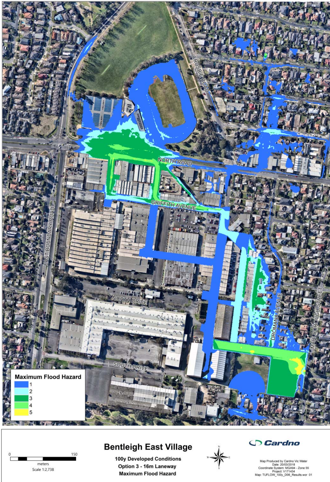
Figure 7-21 1% AEP Maximum Flood Hazards (Option 3)
