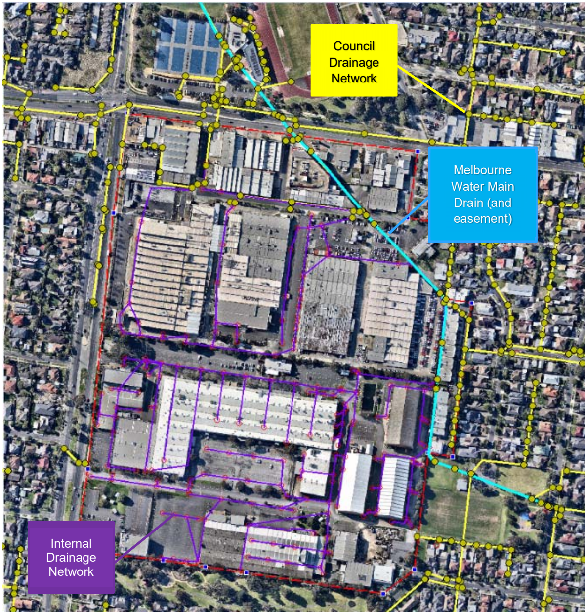
Figure 2-1 Pits and Pipe Network within the hydraulic model
