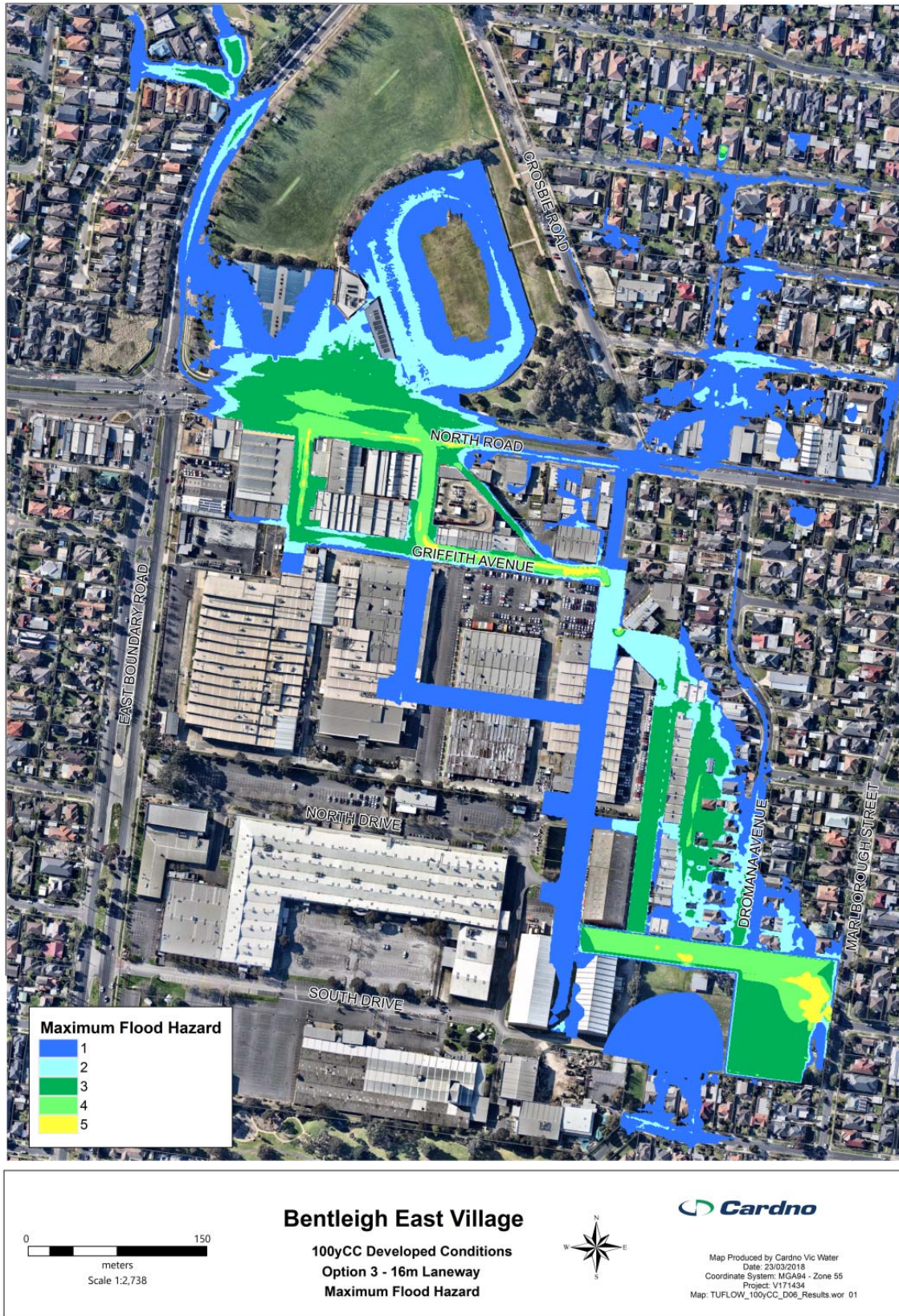
Figure 7-23 1% AEP Climate Change Maximum Flood Hazards (Option 3)
