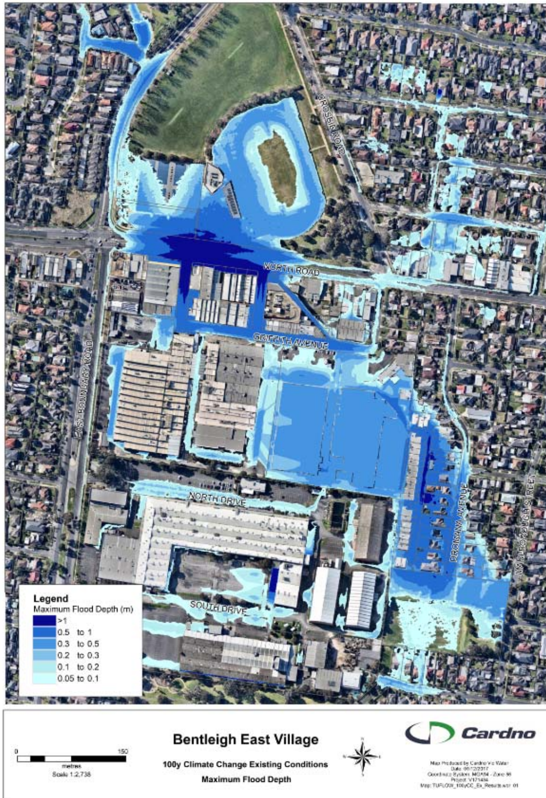
Figure 3-5 1% AEP Climate Change Maximum Flood Depths (Existing Conditions)
