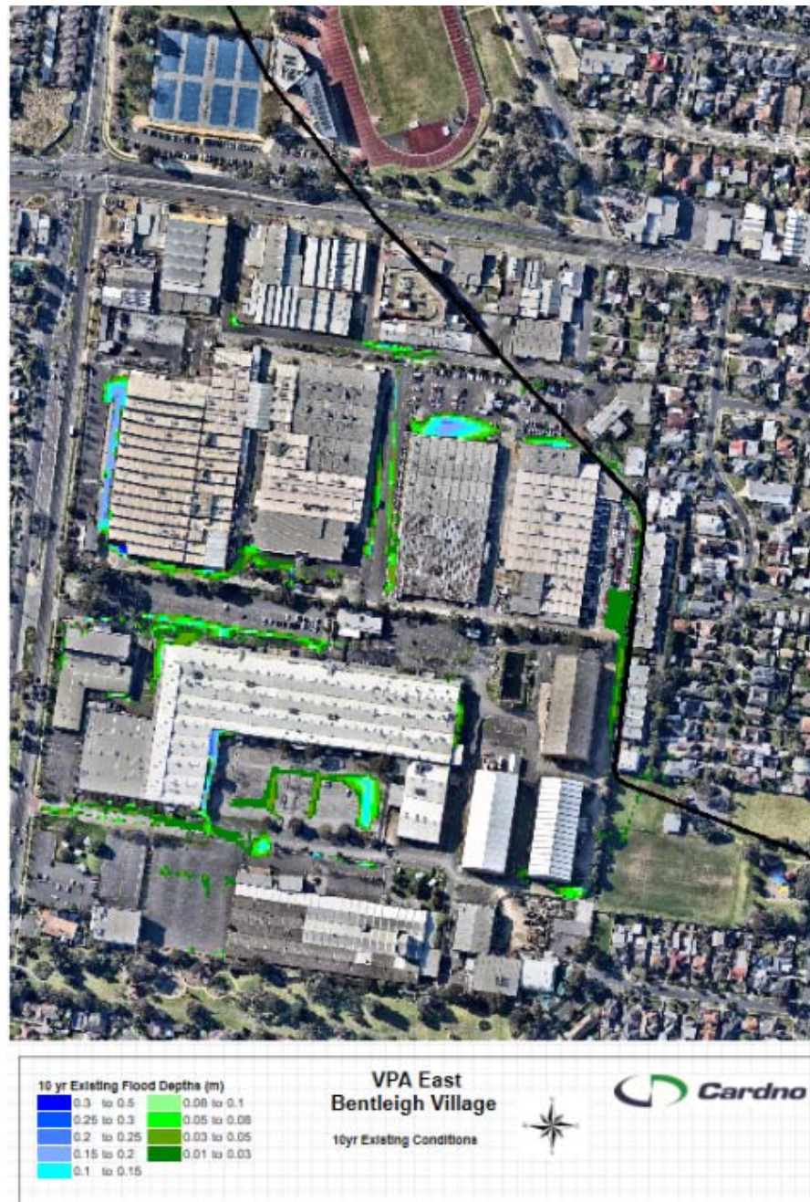
Figure 3-2 10% AEP events existing conditions depth plot
