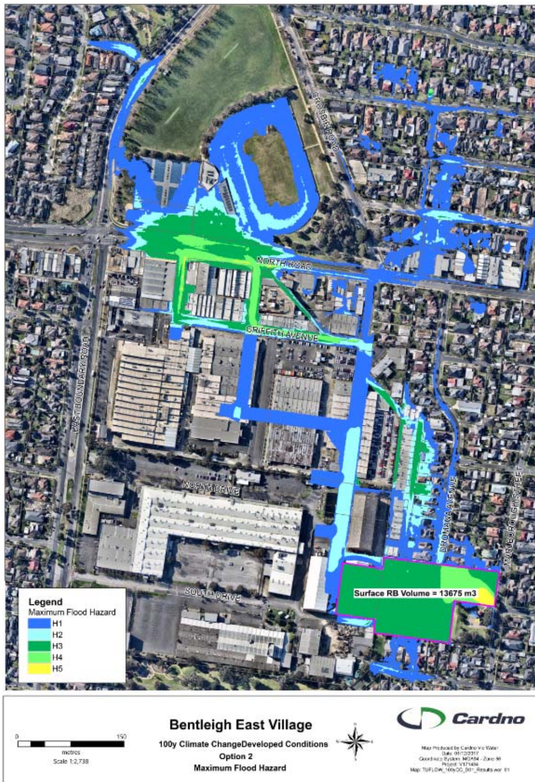
Figure 7-14 1% AEP Climate Change Maximum Flood Hazards (Option 2)
