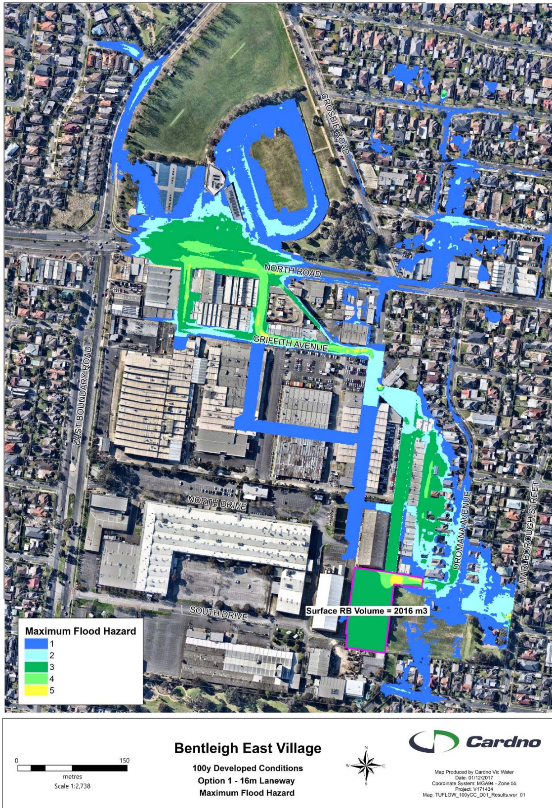
Figure 7-5 1% AEP Maximum Flood Hazards (Option 1)
