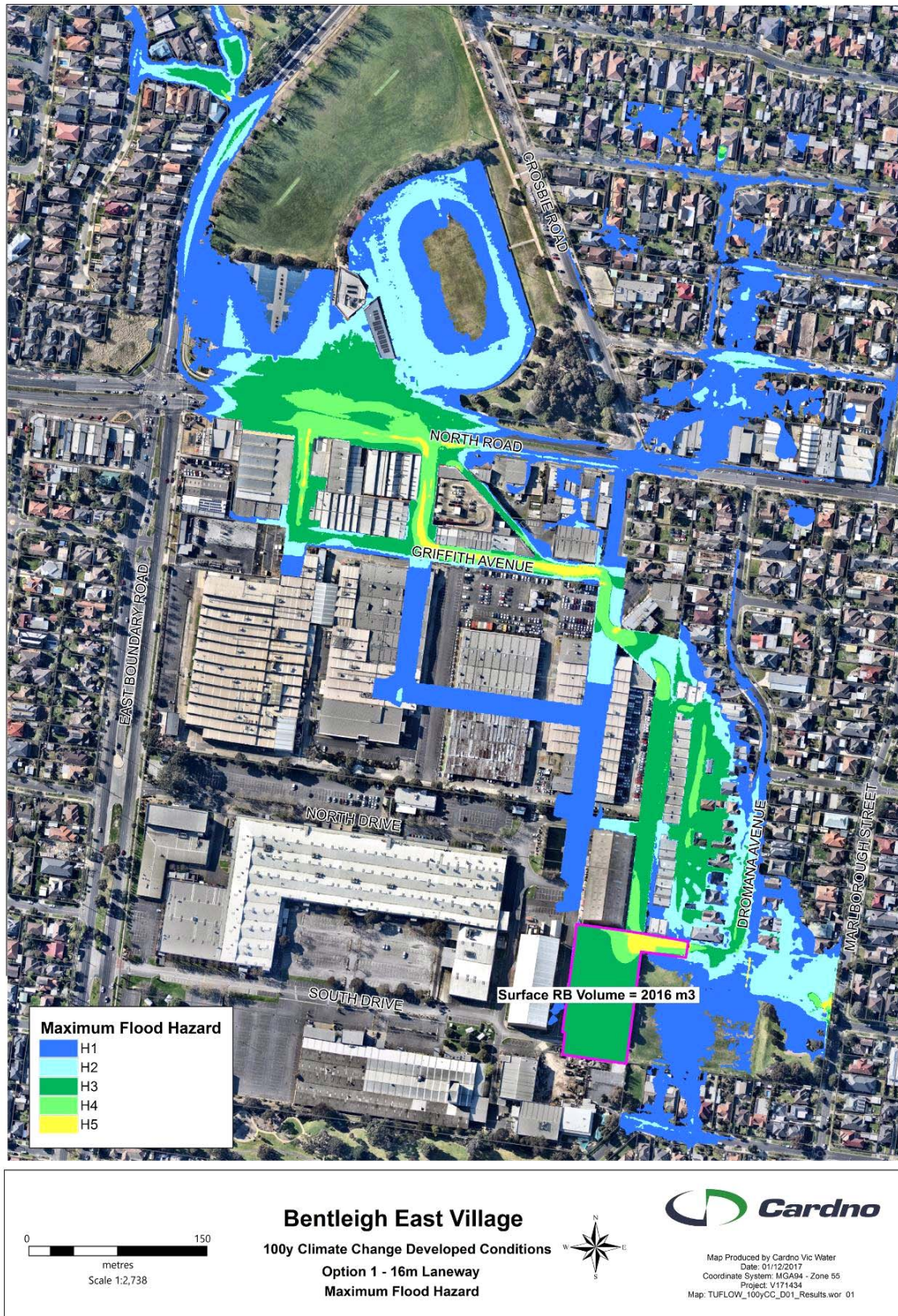
Figure 7-7 1% AEP Climate Change Maximum Flood Hazards (Option 1)
