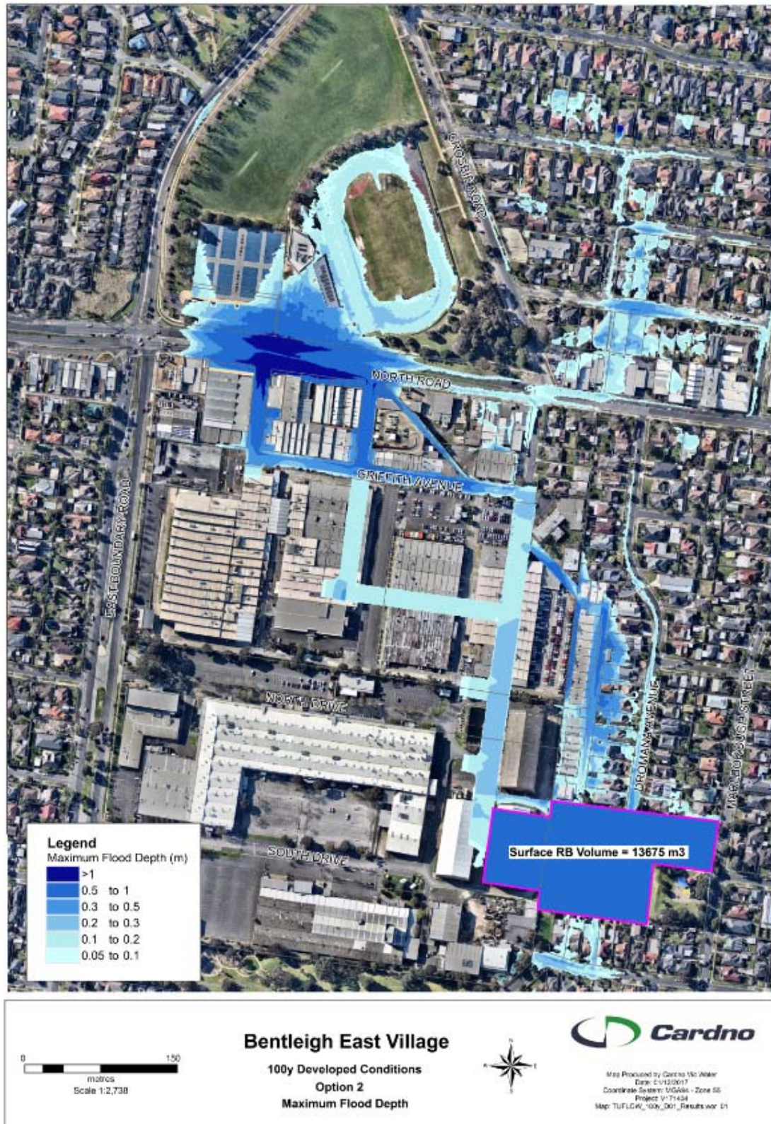
Figure 7-11 1% AEP Maximum Flood Depths (Option 2)
