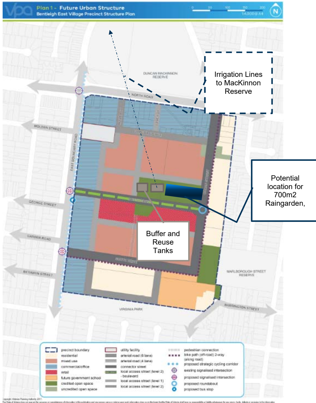
Figure 10-4 Option B Stormwater harvesting and reuse Scheme location
