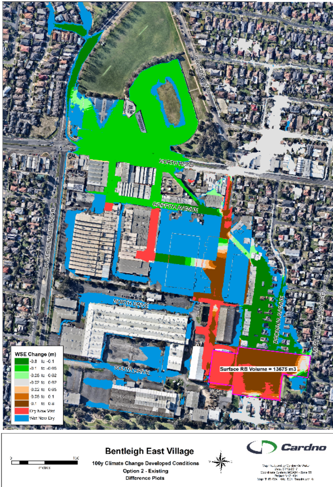
Figure 7-10 1% AEP Climate Change Difference Plot (Option 2)
