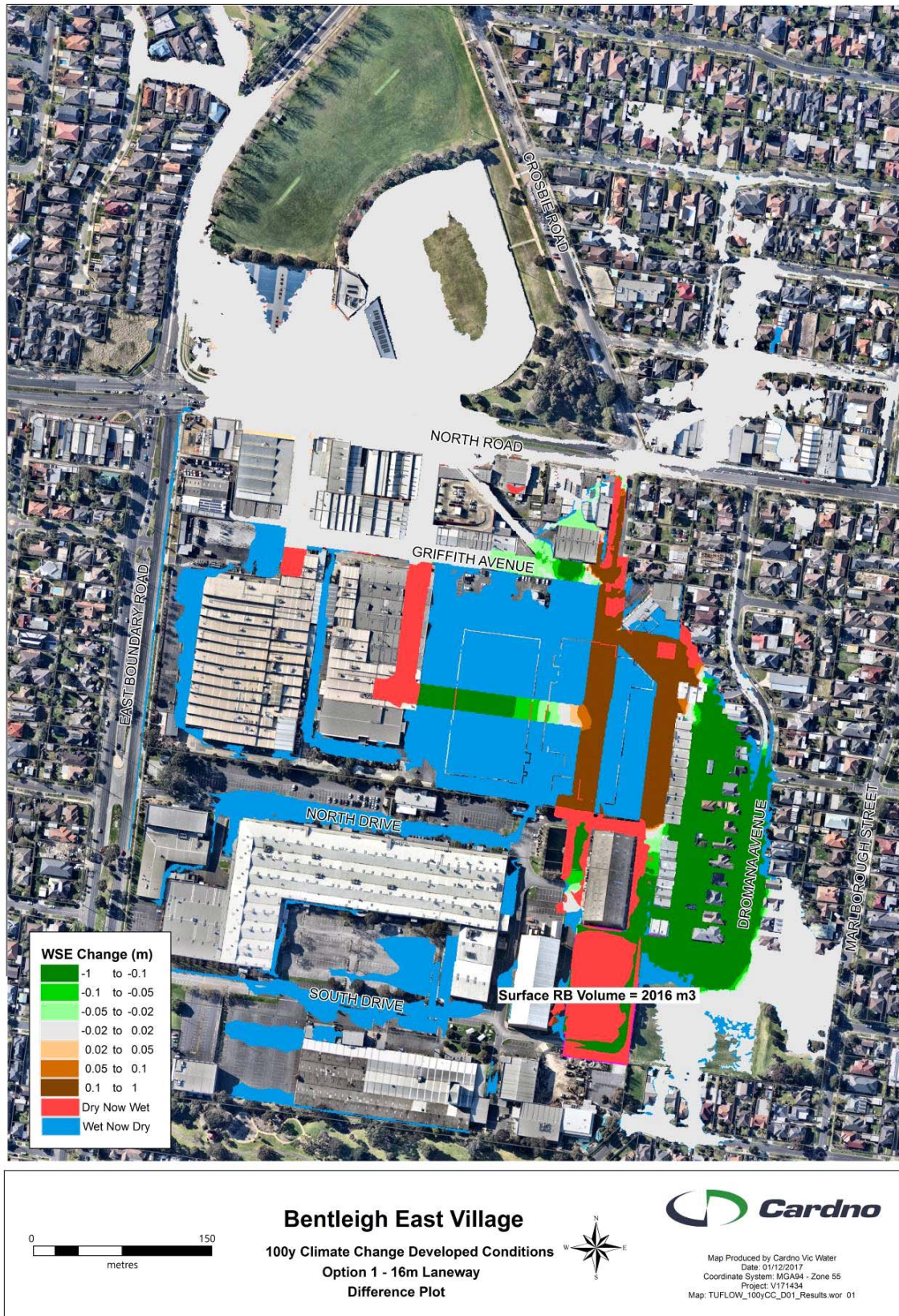
Figure 7-3 1% AEP Climate Change Difference Plot (Option 1)
