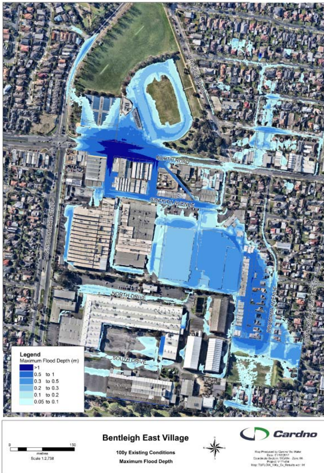
Figure 3-3 1% AEP Maximum Flood Depths (Existing Conditions)
