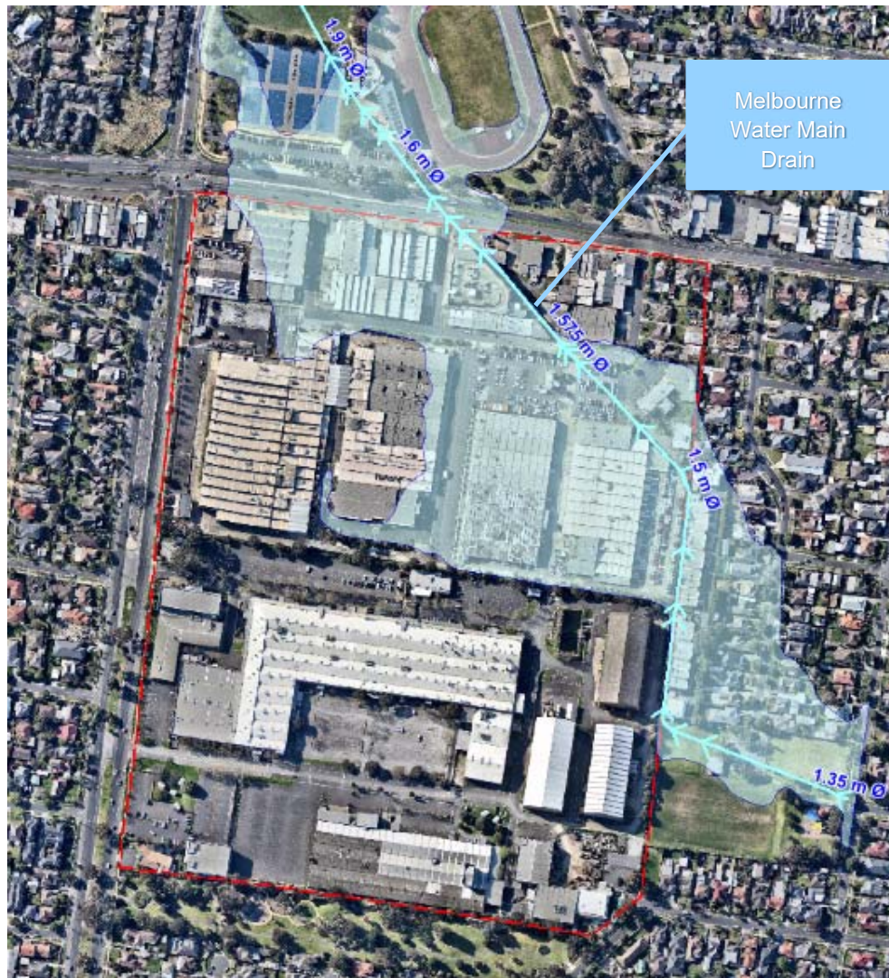
Figure 2-2 Melbourne Water 1% AEP flood map for the EV site
