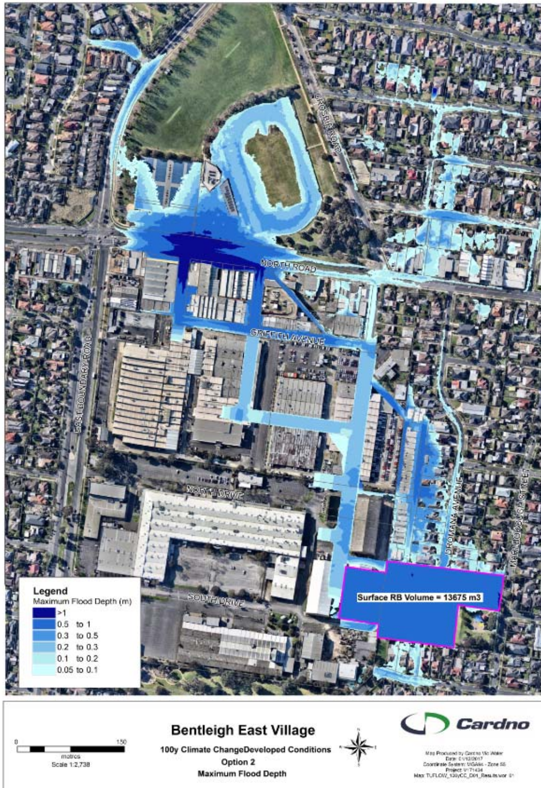
Figure 7-13 1% AEP Climate Change Maximum Flood Depths (Option 2)
