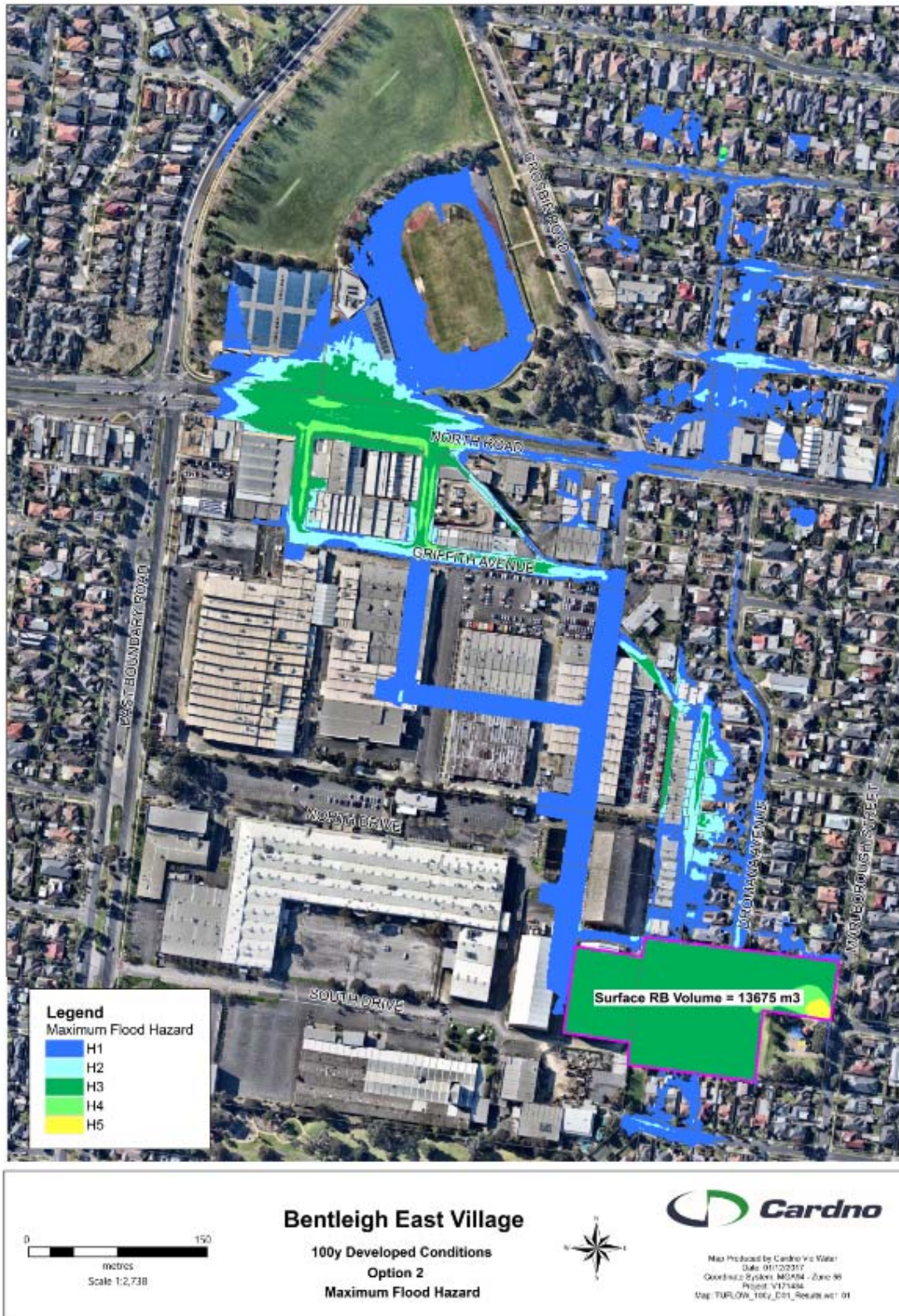
Figure 7-12 1% AEP Maximum Flood Hazards (Option 2)
