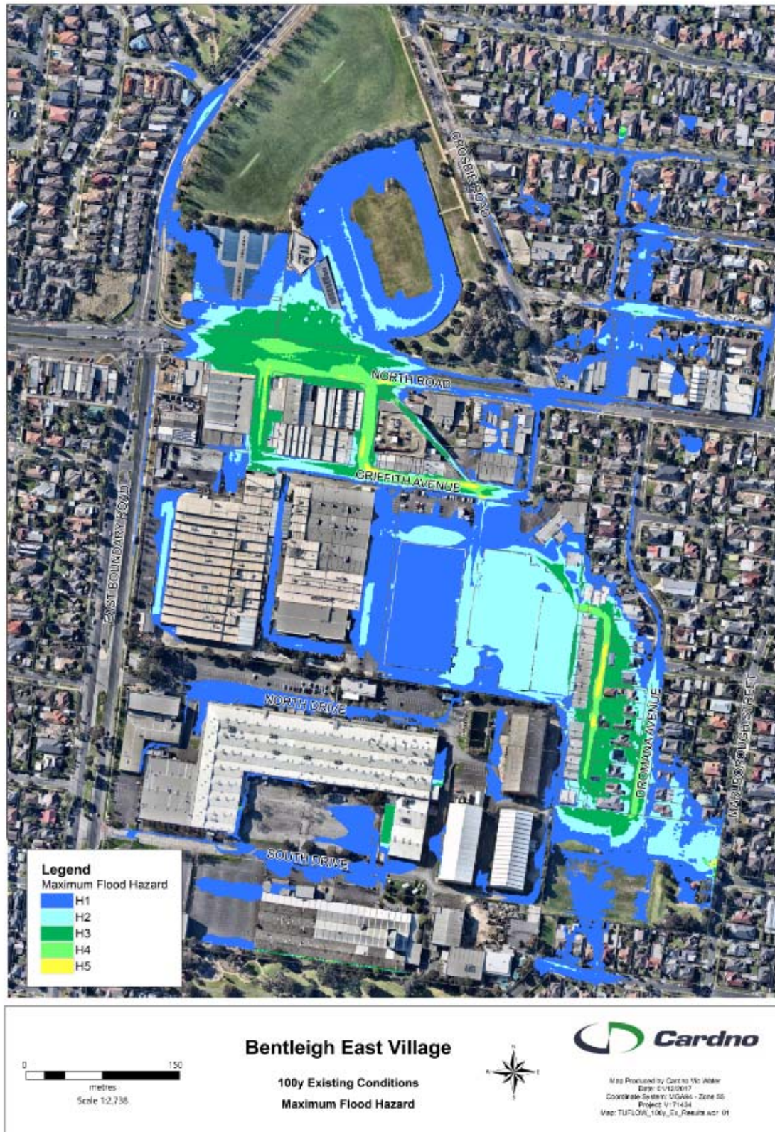
Figure 3-4 1% AEP Maximum Flood Hazards (Existing Conditions)
