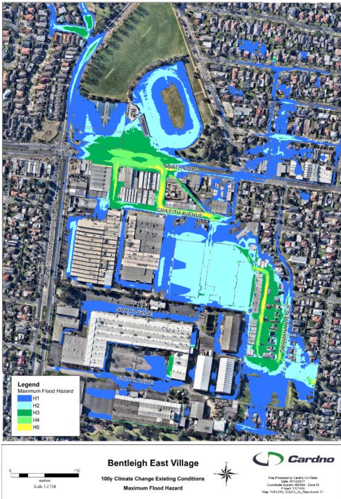
Figure 3-6 1% AEP Climate Change Maximum Flood Hazards (Existing Conditions)
