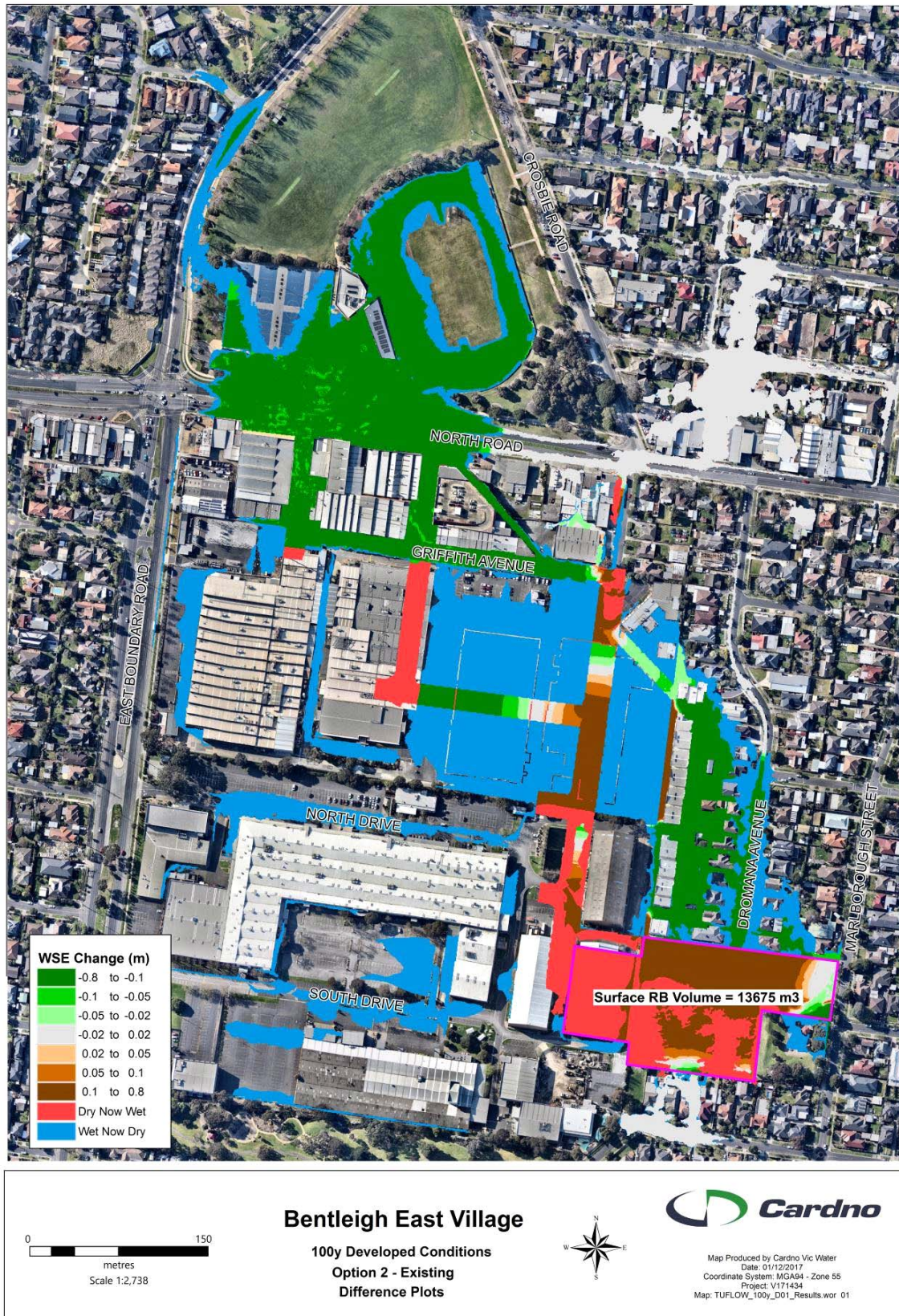
Figure 7-9 1% AEP Difference Plot (Option 2)
