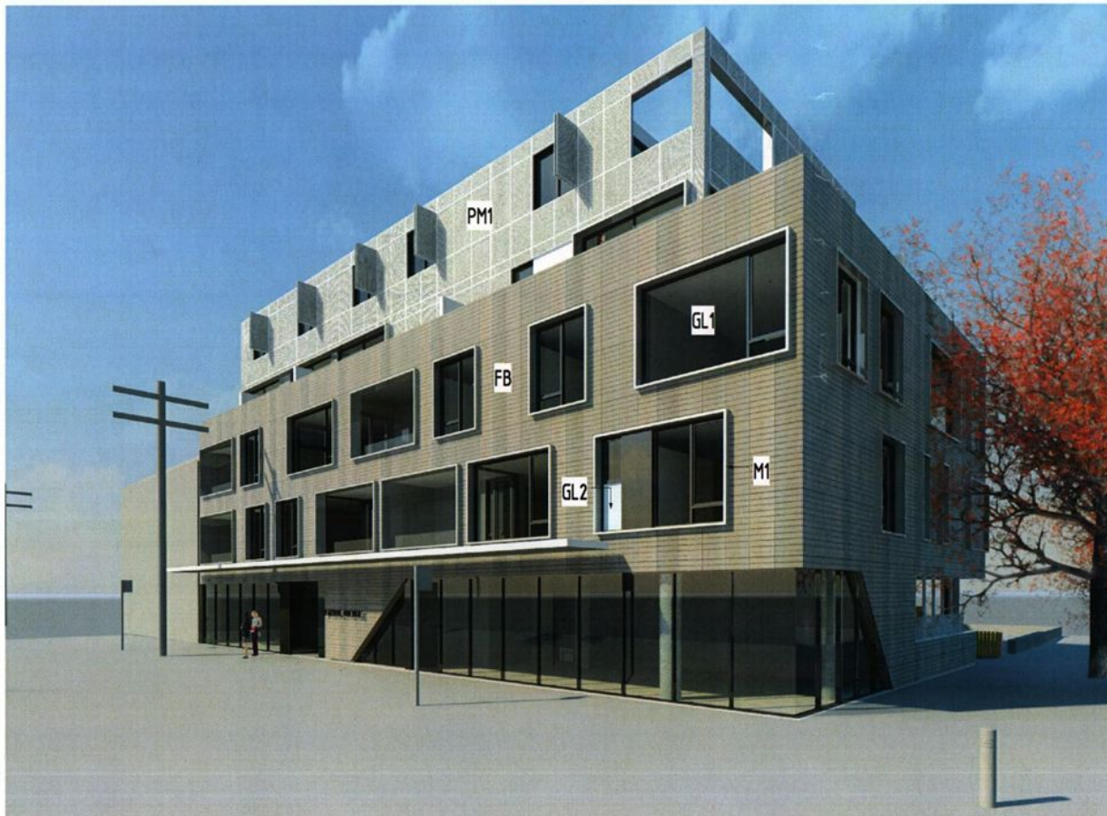
GL1 CLEAR GLAZING IN POWDER COATED ALUMINUM WINDOW FRAMES COLOUR - DALUX ZEUS CHARCOAL
