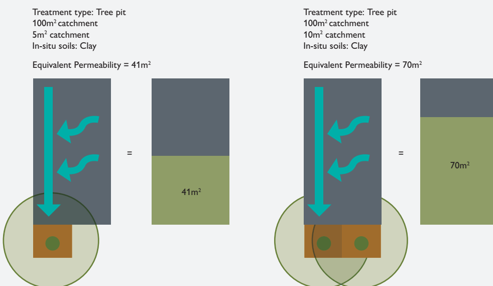
Figure 18. Equivalent permeability provided by WSUD tree pits 14
